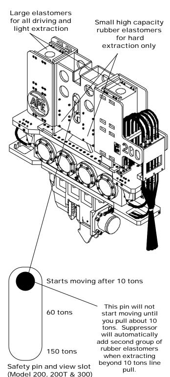
The APE vibro suppressor has two sets of rubber elastomers. One set is very large and is used only for driving and very light extraction. On most light duty jobs, only the large elastomers will be engaged and the vibro will operate very smooth.
